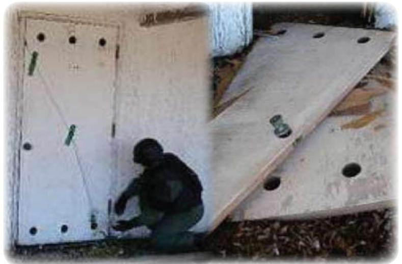
Outward opening solid particle core door. Hinge charge used for a diagonal shot while on target. Shot functioned as designed and separated the top of door from the bottom.
