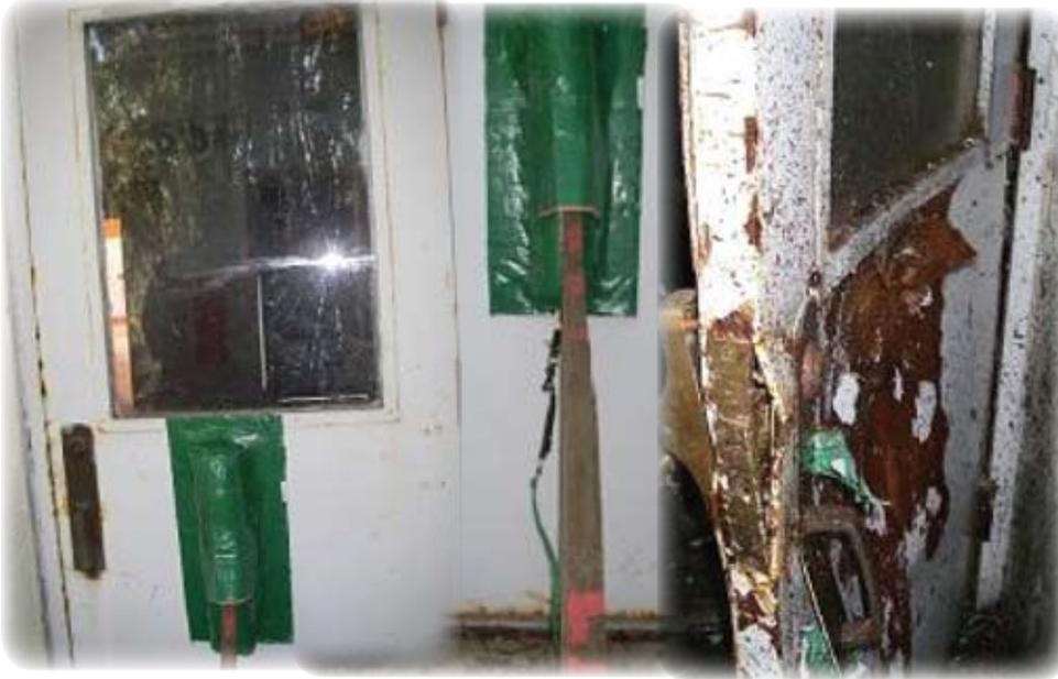
Water impulse shot used on an outward opening metal skin over solid wood fire door with Plexiglass window. The shot defeated the door and did not break the window in the door. The window above the door was cracked and a window adjacent to the door was broken. No other collateral damage. –Training shot
