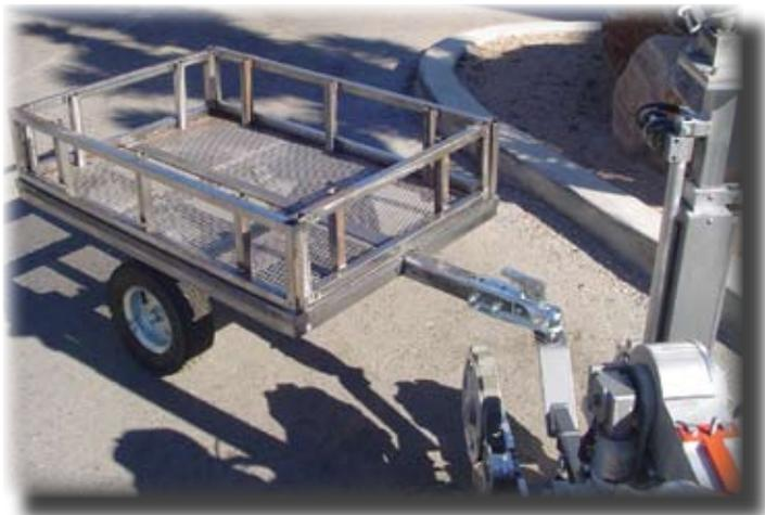
REMOTEC F6A with stake bed trailer featuring removable sides and interchangeable top deck
