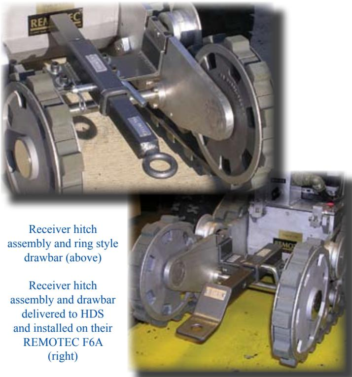
Receiver hitch assembly and ring style drawbar (above)
