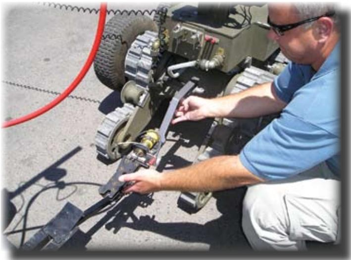
Drawbar for the “Quick Release” system designed to leave the trailer behind (commonly used with LVB delivery systems)
