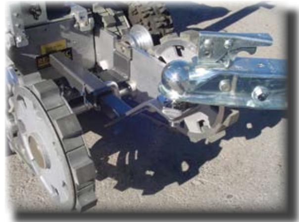
Close-up of the F6A Hitch system with ball hitch drawbar
