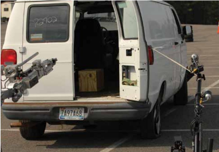
interior door, locate the suspicious item and remove it to a containment vessel. This was a low-light situation requiring the use of lights or night vision on the robot.
