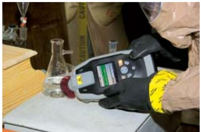
The FirstDefender Raman spectrometer is used to analyze an unknown chemical through the glass without touching or moving the sample.
