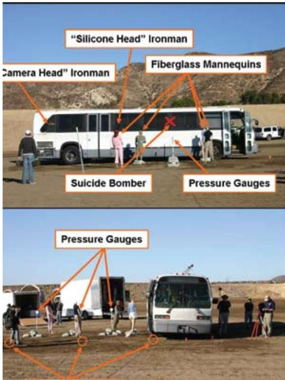
Figure 4. Bus Exterior Before Explosion
